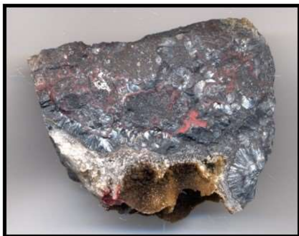
Figure 40. Massive stibnite with cinnabar (red) filling voids and fractures. Note the dark steel-gray matrix color, typical of rocks rich in stibnite.
