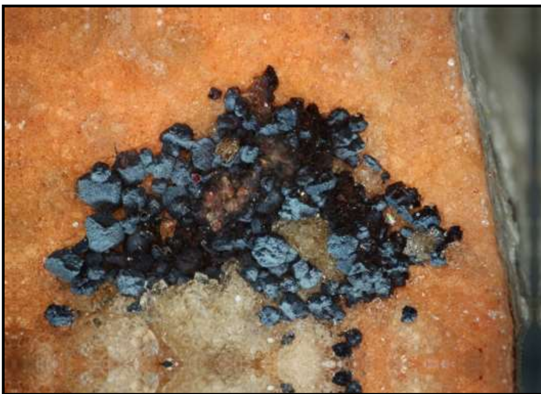
Figure 76. A group of prior cinnabar crystals replaced by corderoite on a quartz base. FOV = 1 mm. The crystals are coated (or replaced) with a dark gray/metallic phase have been identified as cinnabar. The core of these crystals are hollow with a highly reflective silvery phase, which was identified as corderoite. The crystals range in size from 0.5 to less than 0.1 mm. Some crystals show a pyramidal termination, while others show no crystal forms.
