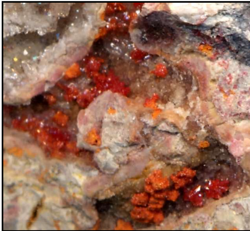
Figure 142. Sample showing grouping of terlinguacreekite crystals on matrix. FOV = 15 mm.
