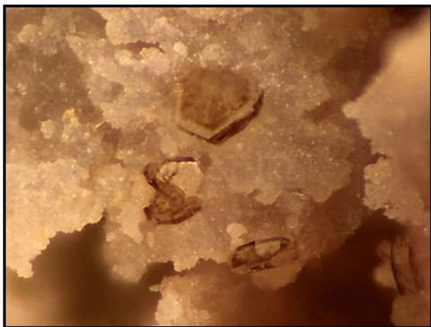
Figure 253. View of four tridymite pseudohexagonal crystals on quartz. FOV = 1 mm.
