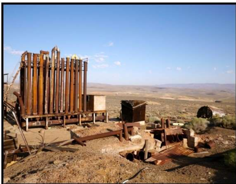
Figure 19. Furnace condensers and retort remains at the Ruja mine (after Blumenfeld 2014)
