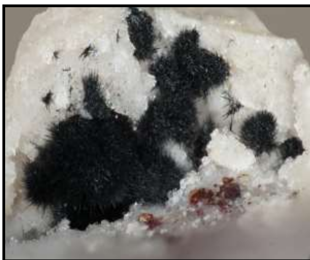
Figure 211. Fine, acicular crystals of cryptomelane in a quartz cavity. FOV = 2 mm.
