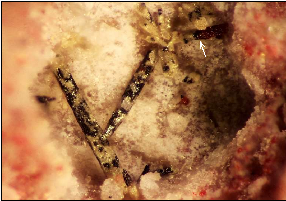
Figure 166. Several prisms of MCDUK-3 on quartz. Note dark zones along the prism length and deep red tip on one prism (arrow). FOV = 1 mm.
