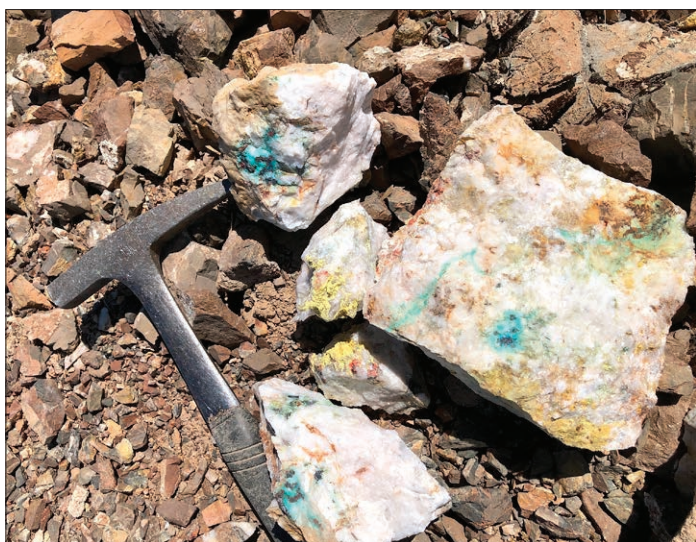
Figure 24. Green staining indicates evidence of secondary copper mineralization in massive quartz; yellow antimony oxide mineralization is also present, field of view 38 cm.
